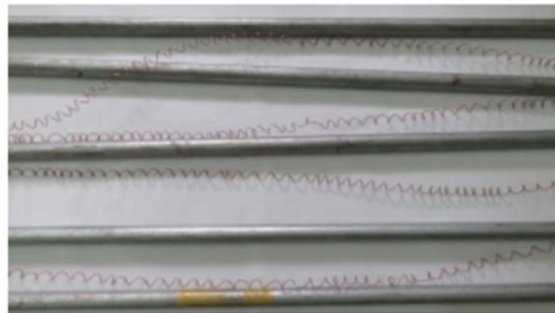
Fig. 3.4: Pipes with Agitator
