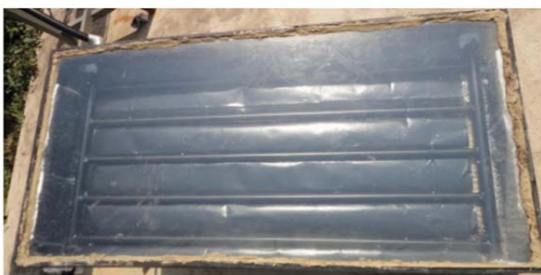
Fig. 3.3: Absorber plate with pipes
